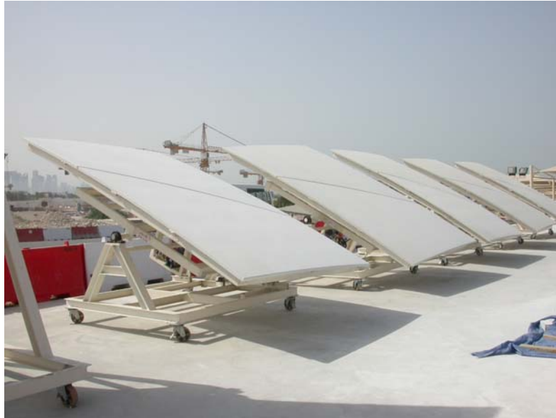
Figure 10 : Mock-up of the cladding panels
