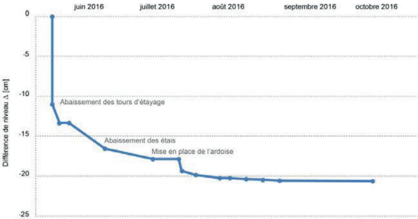
Figure 11: Evolution of the vertical displacement of the end of the cantilevered northern roof
