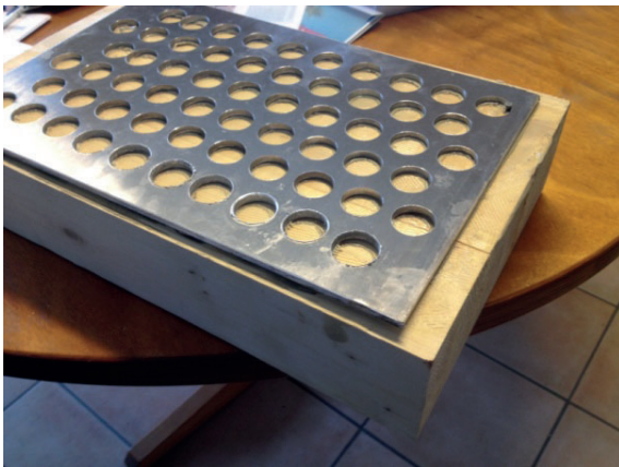
Figure 3: Delamination of the aluminum plates observed after the tests
