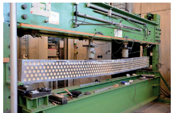
Figure 5: photo of the laboratory experiment on a hybrid wooden-steel beam
